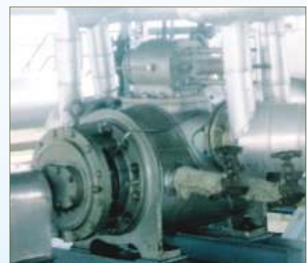
Twin Screw Pump pumping Bitumen at a facility in Tehran, Iran
